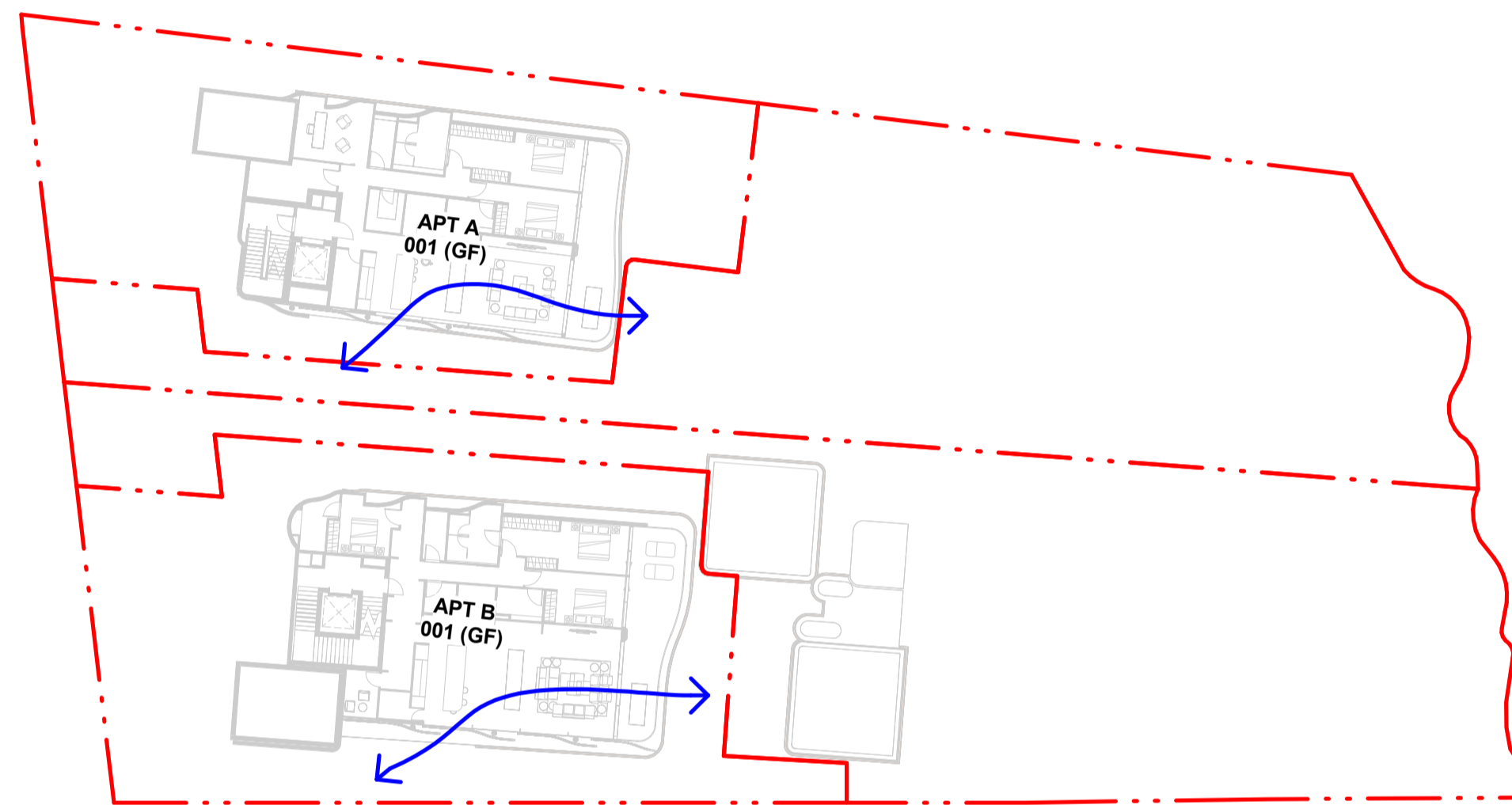
LEVEL R4 GROUND - CROSS VENTILATION (2/2)
