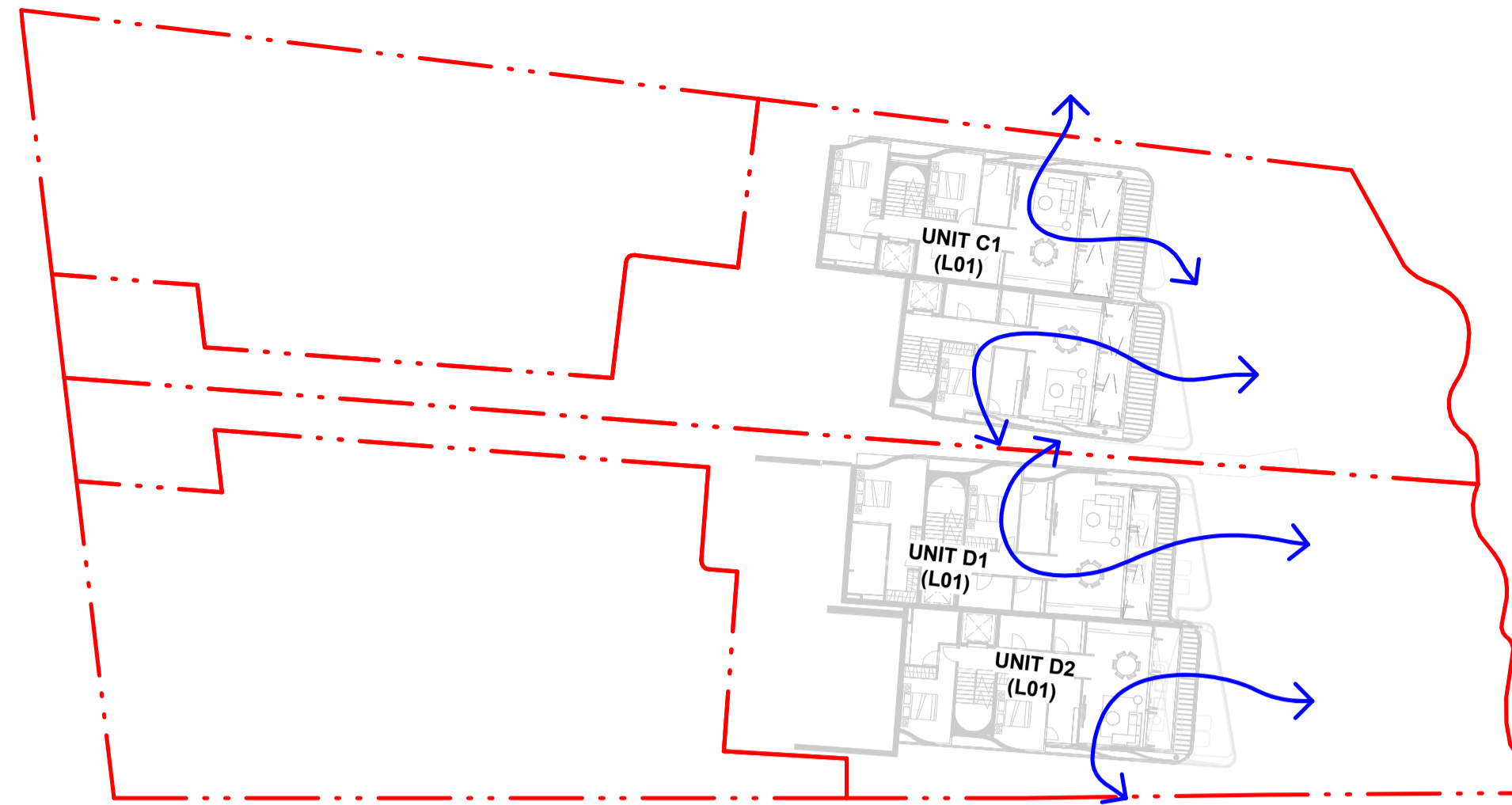
LEVEL R2-L01 - CROSS VENTILATION (4/4)
