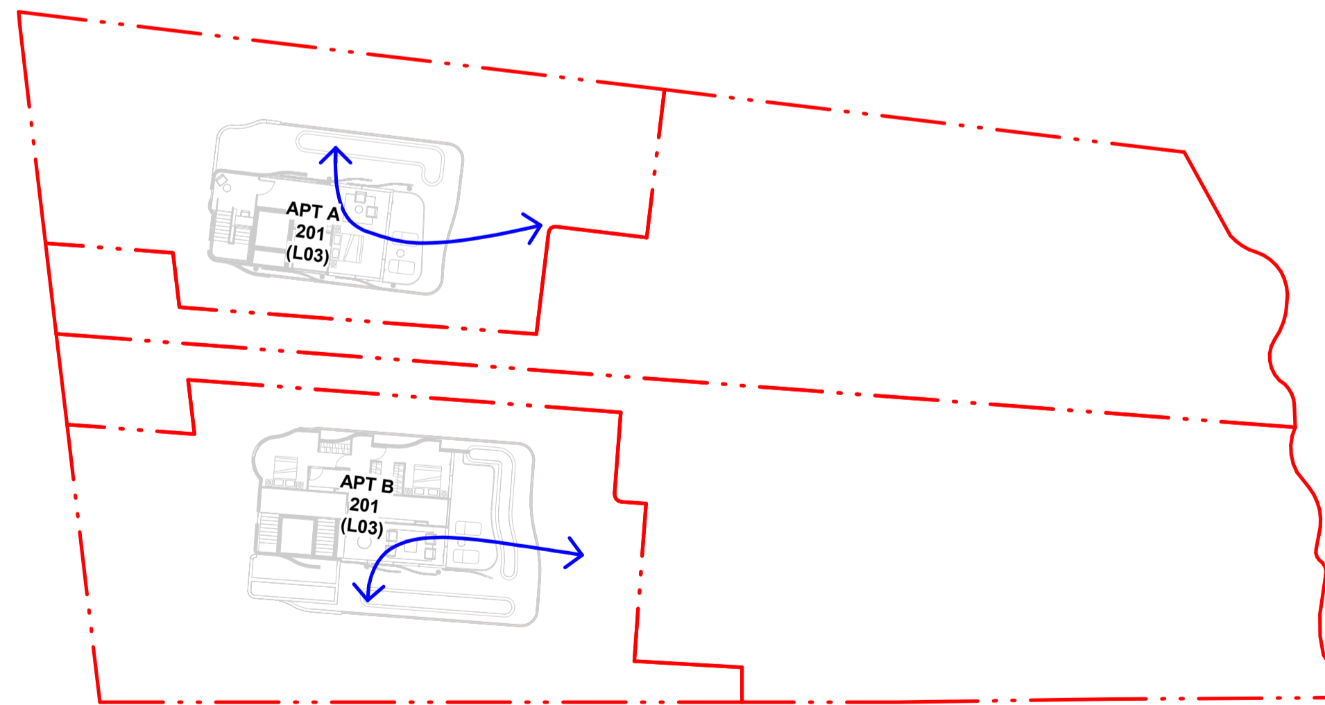
LEVEL R4-L03 - CROSS VENTILATION
