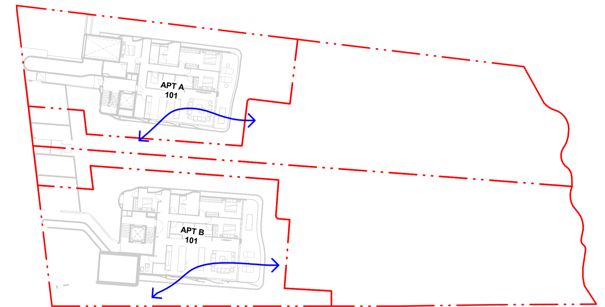
LEVEL R4-L01 - CROSS VENTILATION (2/2)
