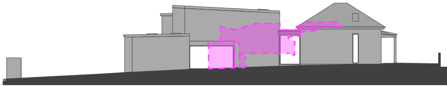
3PM-PROPOSED SHADOW MID WINTER 1:200 @ A3 ADDITIONAL SHADOW AS INDICATED NOTE: EXISTING FENCE & 3M HIGH BOUNDARY SCREEN PLANTING NOT PLOTTED.
