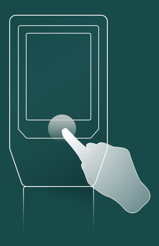
To wake the meter touch the "Touch here to start" button near the green flashing light. Now touch anywhere on the screen to begin.
