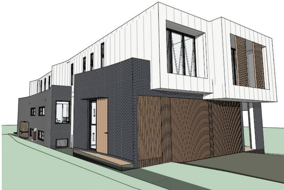
Front and western elevations with the second unit's front door to the side, to assist the building appear from the street as a single dwelling (Design Corp Architects).
