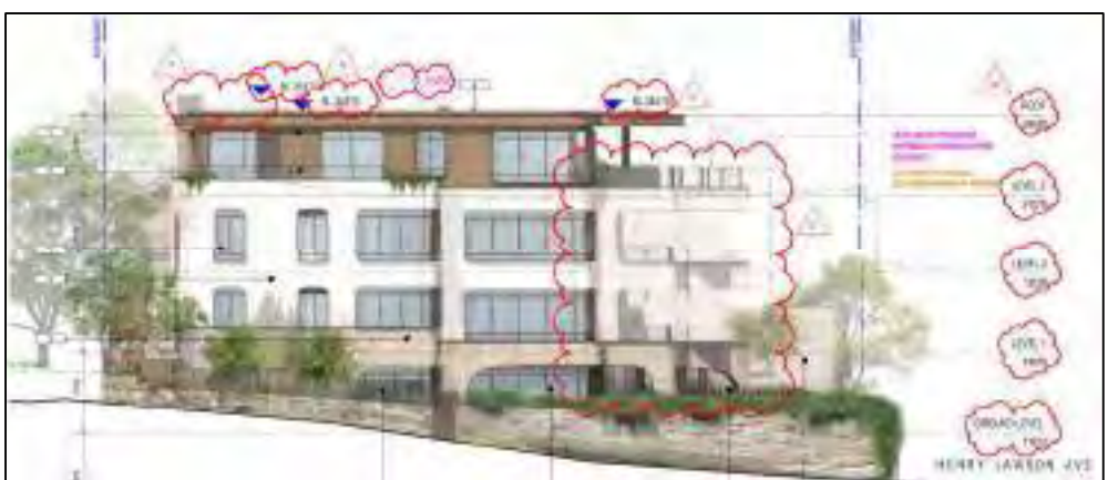
Figure 7: Extract of west elevation (Blues Point Road) showing LEP 8.5m height line (Source: Squillace Architecture, Project No. HIG2307, Sept 2024)
