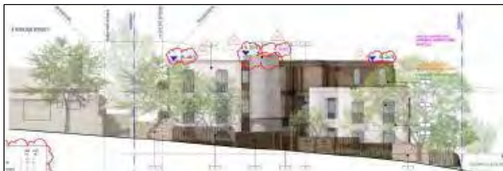
Figure 4: Extract of north elevation (Warung St) showing LEP 8.5m height line (Source: Squillace Architecture, Project No. HIG2307, Sept 2024)
