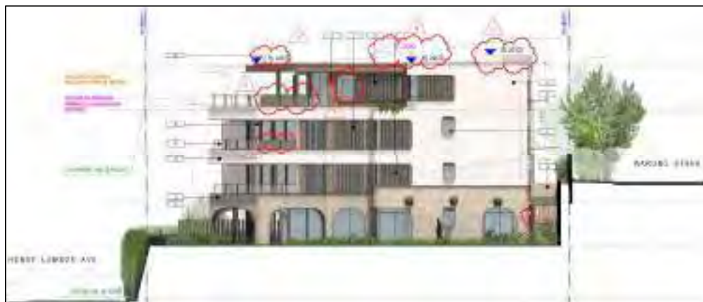
Figure 6: Extract of east elevation (from No. 3 Warung St) showing LEP 8.5m height line (Source: Squillace Architecture, Project No. HIG2307, Sept 2024)
