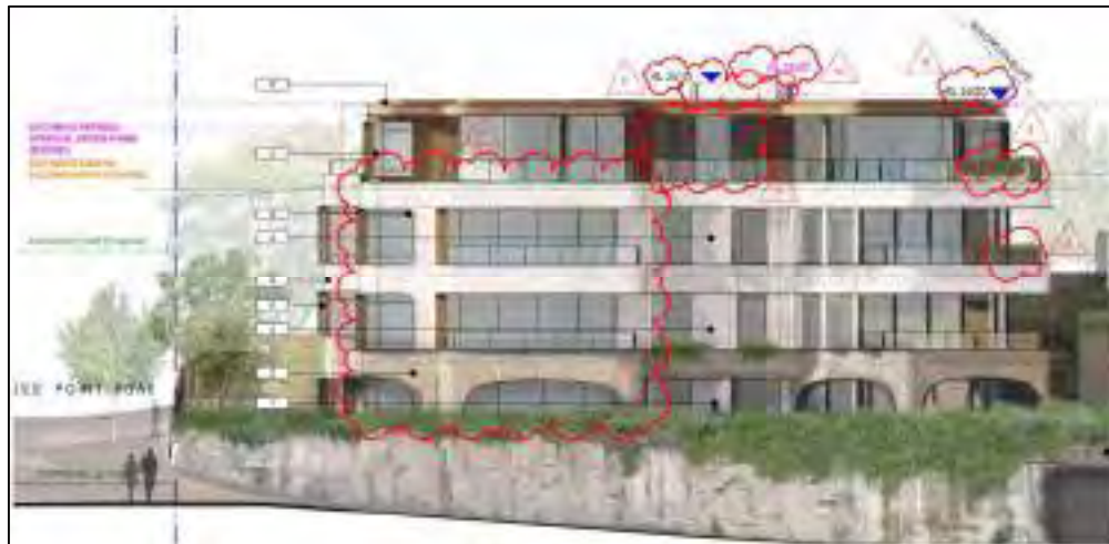
Figure 5: Extract of south elevation (Warung St frontage) showing LEP 8.5m height line (Source: Squillace Architecture, Project No. HIG2307, Sept 2024)
