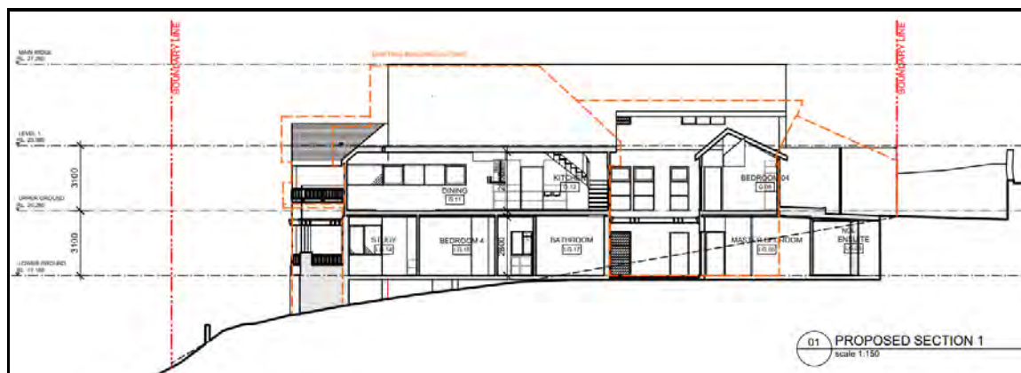
Figure 20: Section of building showing the existing building outline against the proposed building outline.
