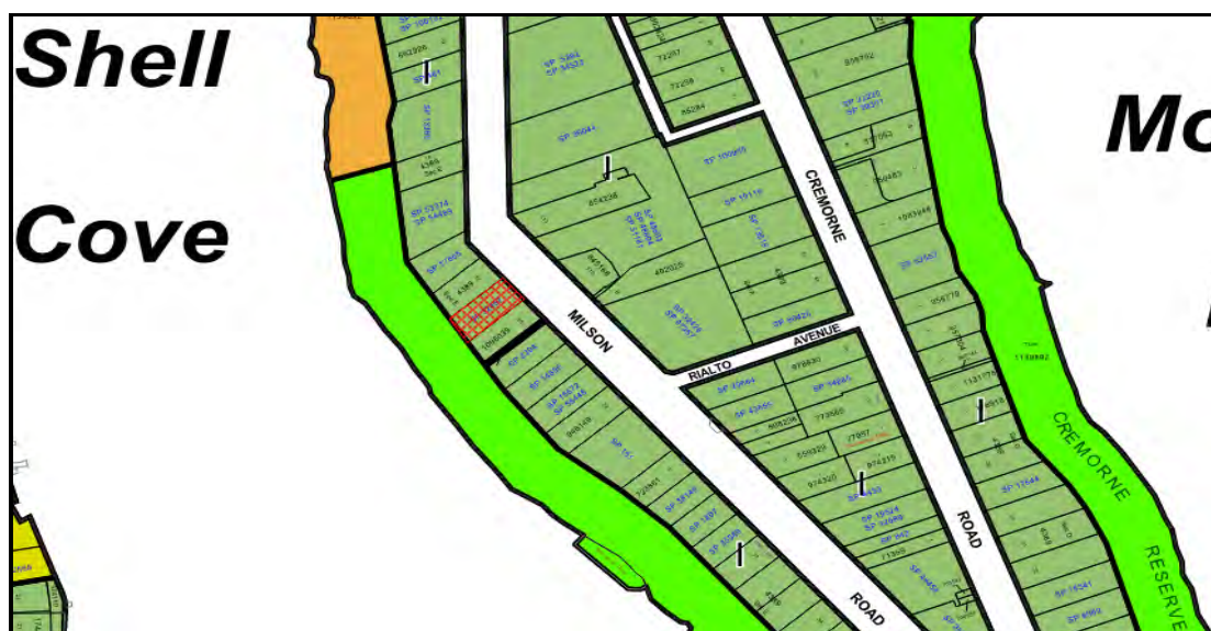
Figure 19: Maximum Building height map (green denotes 8.5m maximum) with subject site identified cross hatched in red.
