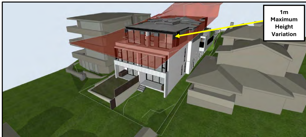
Figure 3: Excerpt Height Plane Diagram, illustrating maximum building height to the northeast corner of the built form.
