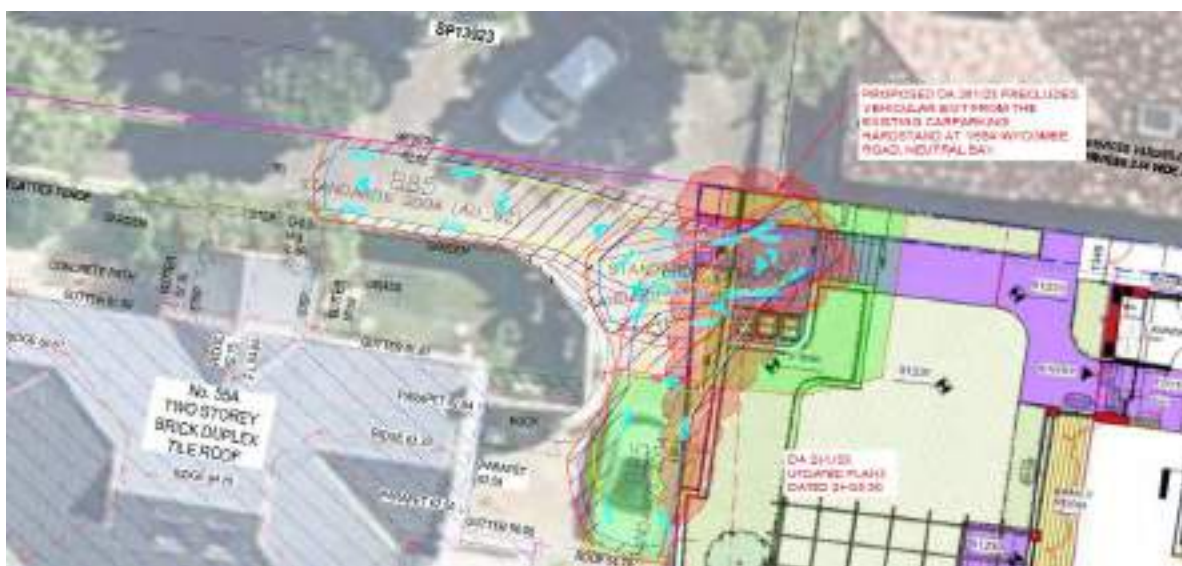
Swept path diagram, from the submission on behalf of the owners of 55A Wycombe Road (Traffix Transport Planners 04 07 24)
