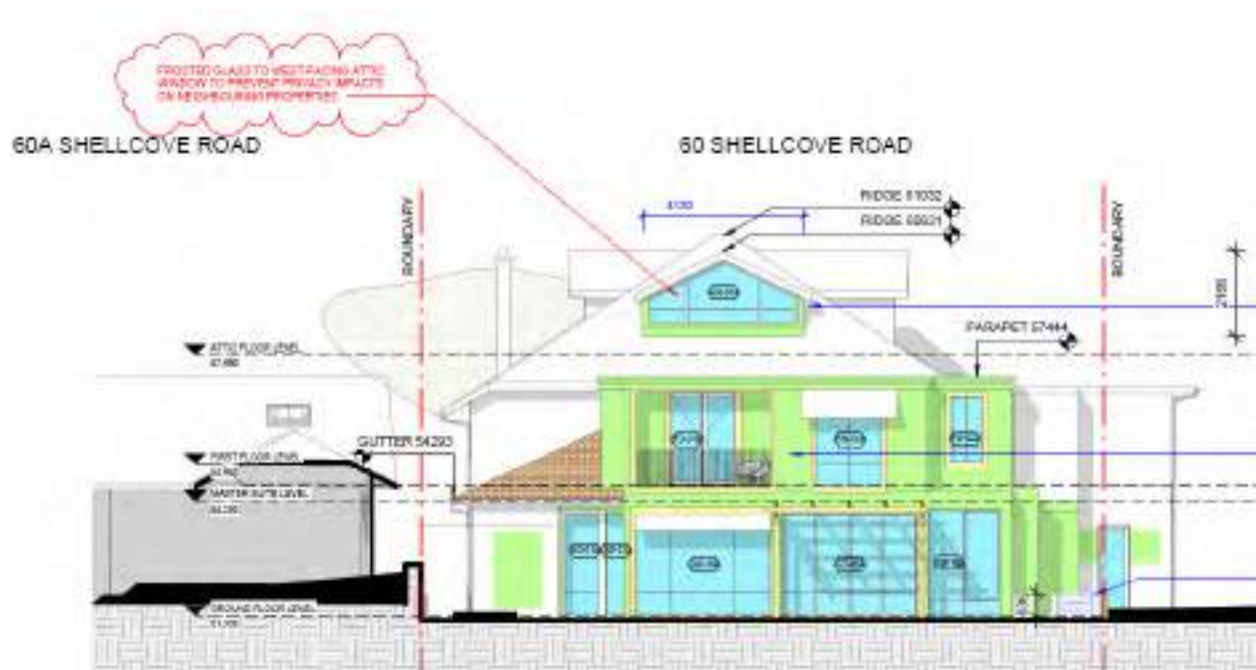
Eastern elevation, alterations coloured (Archer Design).
