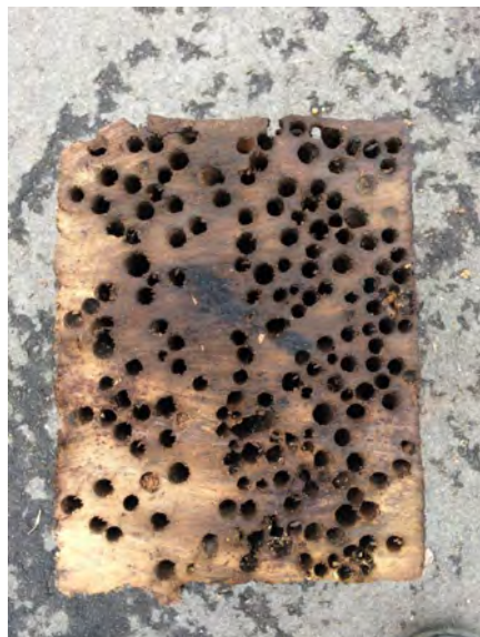
Termites found in timber marine structure
