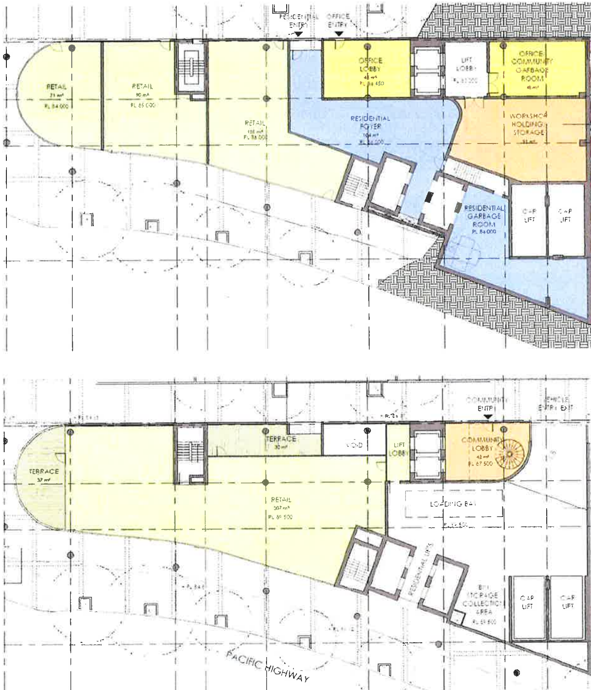
Figure 12 – Lower Ground (top image) and Ground Floor (bottom image) Plans (Concept Design Report, Kann Finch)
