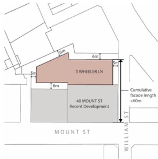
Figure 8A: 1 Wheeler Lane with proposed nil above podium setback to southern boundary
