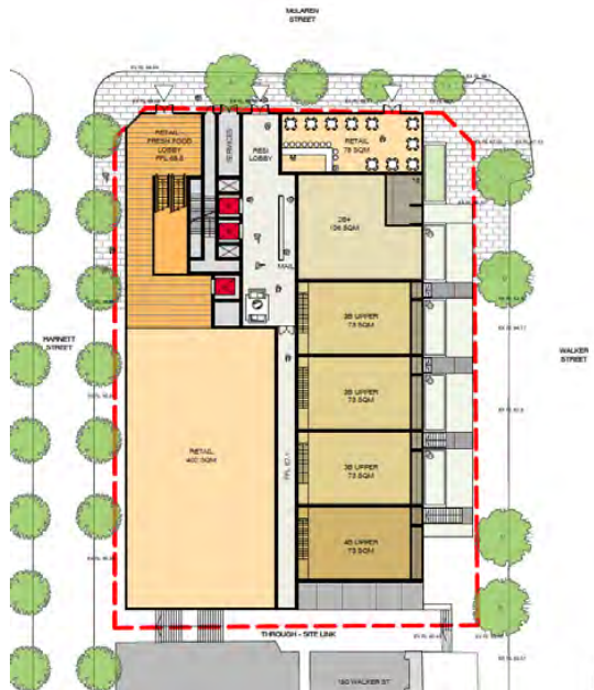
Figure 28: Upper ground floor
