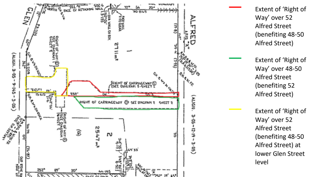
FIGURE 16: Extract from DP738322, depicting the existing 'Right of Carriageway' created pursuant to section 88B of the Conveyancing Act 1919)
