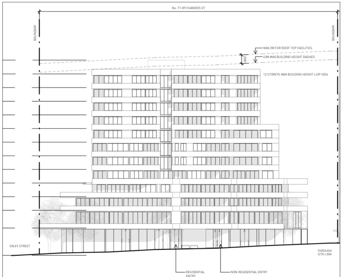
FIGURE 3: Northern (Chandos Street) Elevation Plan, as exhibited (Applicant's amended Architectural Drawings, p. 19)
