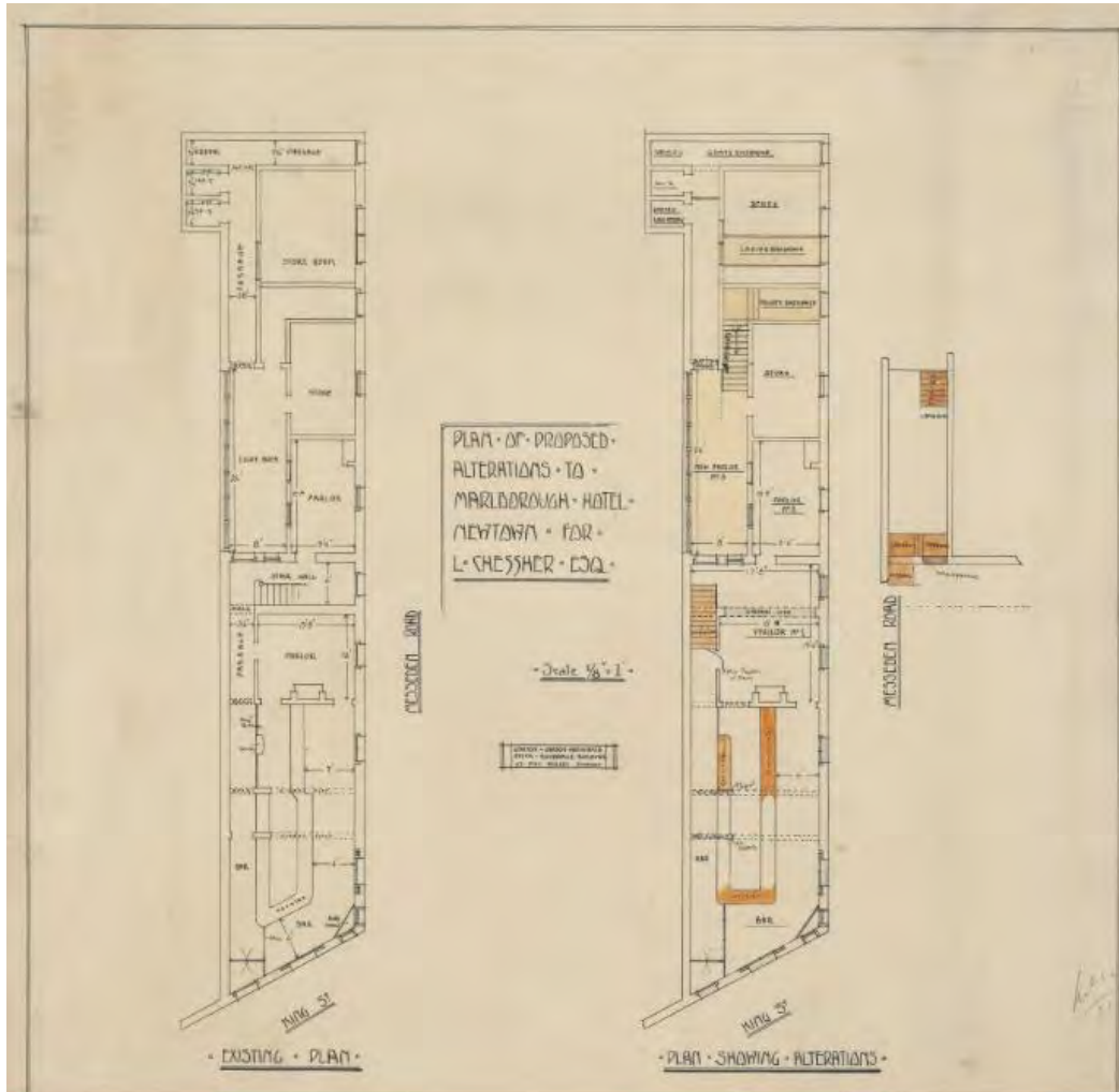
Figure 4.37 Plans for proposed alterations at the Marlborough Hotel, King Street, Newtown (State Archives NSW 1909)
