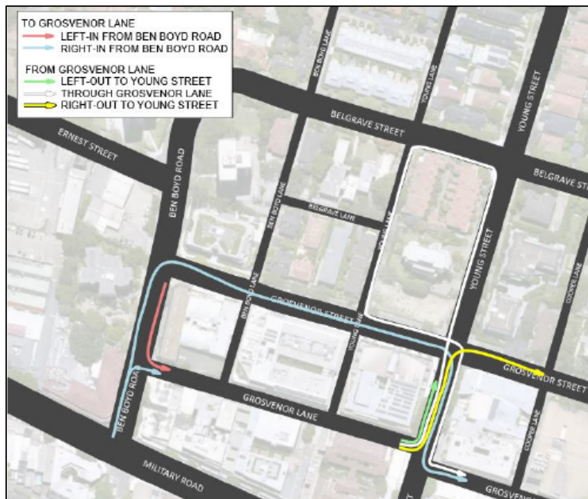
Figure 2: changes to vehicle movements associated with Option 2 - Left Only at Young Street
