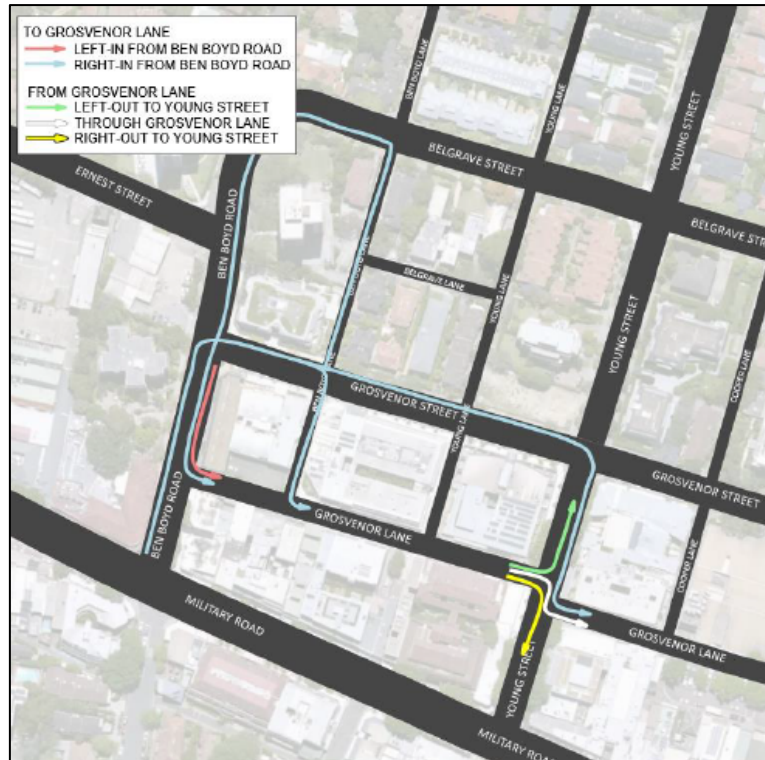
Figure 3: changes to vehicle movements associated with Option 3 - Right turn ban at Ben Boyd Road
