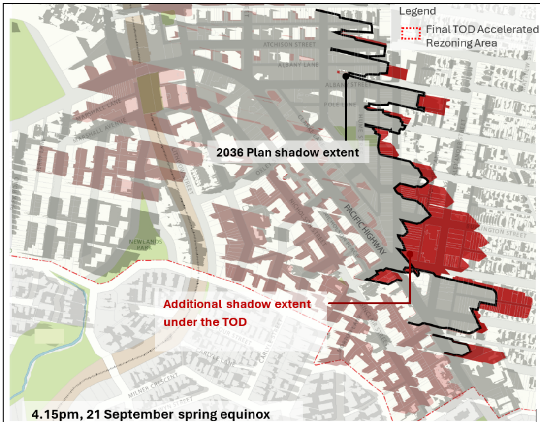
Figure 22 – Shadow diagram at 4.15pm September 21 spring equinox shows the significant increase in lost solar amenity to Crows Nest village under the TOD rezoning compared to the 2036 Plan (Source: NSC)
