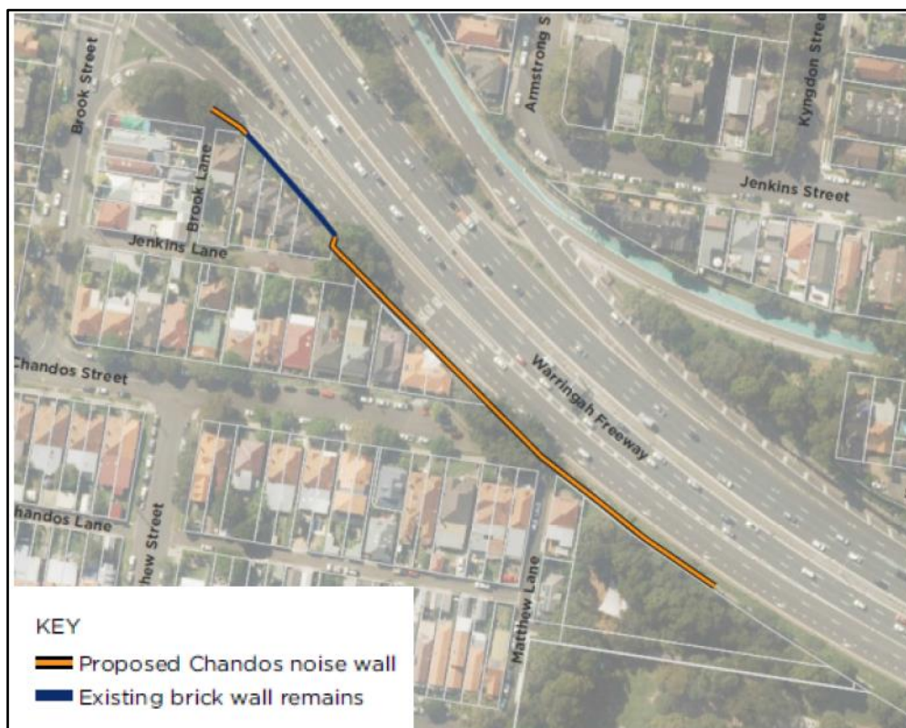
Figure 1- Proposed location of the new RMS Noise Wall adjacent to the Warringah Freeway from Brook Lane to St Thomas Rest Park – approximately 197 metres in length
