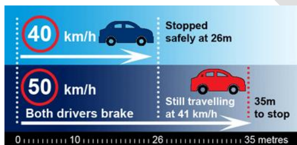
Figure 4. Stopping distances comparison of cars travelling at 40km/h and 50km/h
