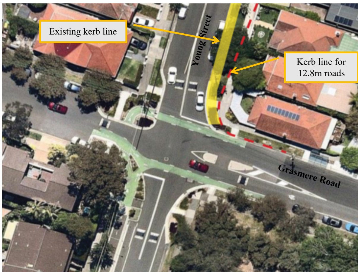
Figure 1 Diagram showing geometric constraints at the intersection between Grasmere Road and Young Street. The section shown in yellow indicates the where the kerb would be located if Young Street was 12.8m wide (the common width across the local road network) and the red line shows where the kerb line would be located if Young Street was 12.8m wide and met Grasmere Road at a right angle. The relative narrowness of Young Street and offset from 90 degrees impact on the type of pedestrian facilities that can be included at the intersection.
