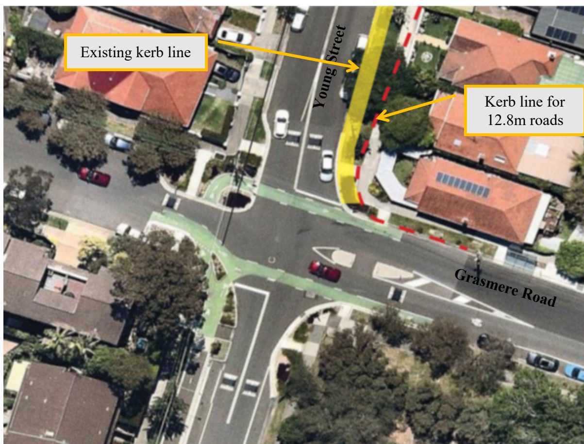
Figure 1 Diagram showing geometric constraints at the intersection between Grasmere Road and Young Street. The section shown in yellow indicates the where the kerb would be located if Young Street was 12.8m wide (the common width across the local road network) and the red line shows where the kerb line would be located if Young Street was 12.8m wide and met Grasmere Road at a right angle. The relative narrowness of Young Street and offset from 90 degrees impact on the type of pedestrian facilities that can be included at the intersection.
