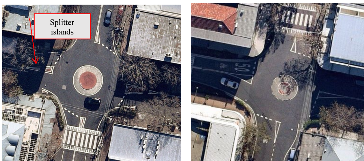
Figure 2 Example of roundabouts with and without splitter islands (Alexander St at Holtermann Street (left) & Alexander St at Burlington St (right) Source: Nearmap
