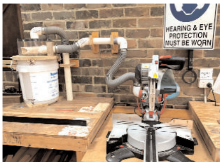
Garry's "Dyson" Dust Extractor for the Drop Saw
