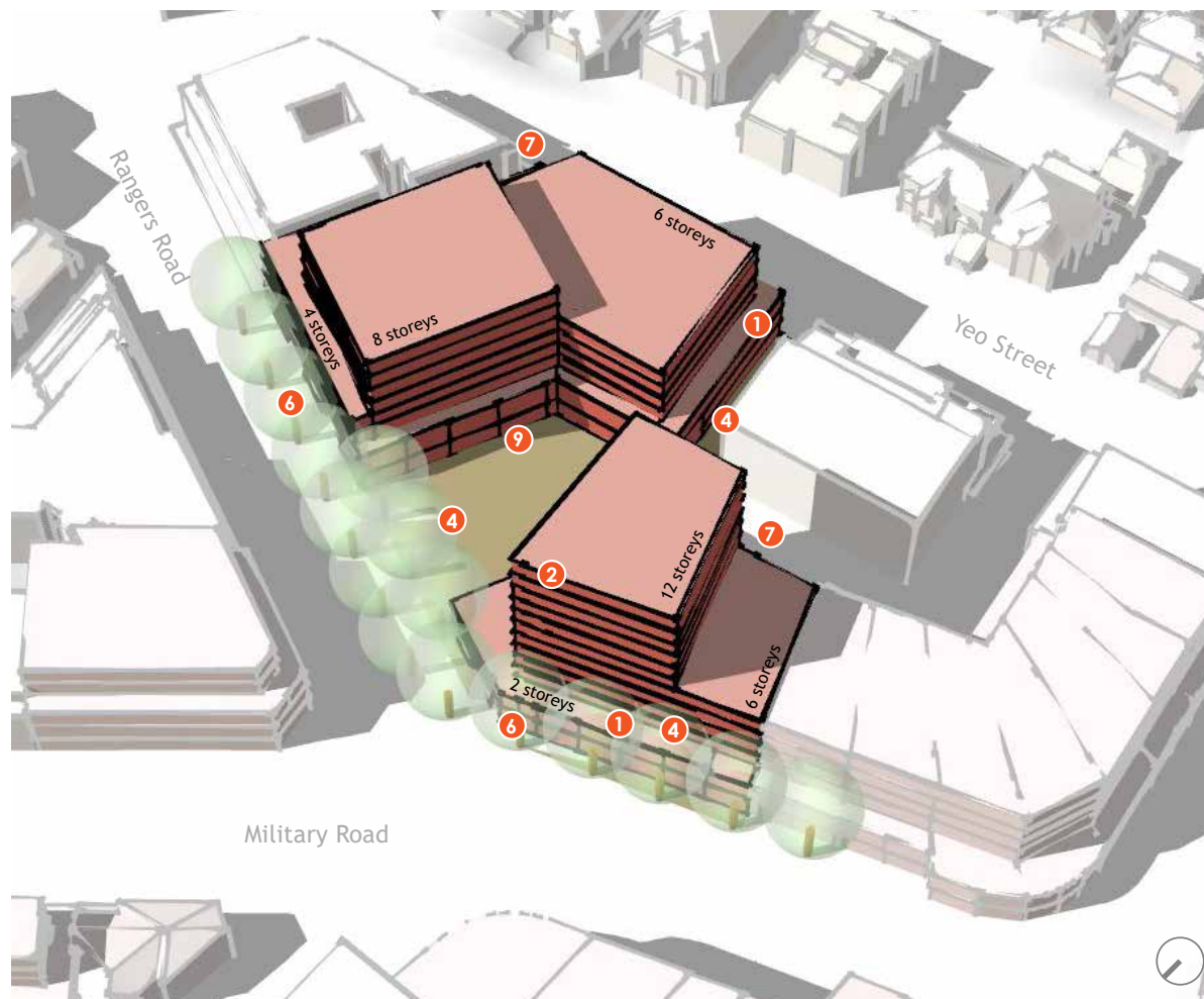
Figure 71 - Illustrative building envelope for Site 3 looking south and showing the new public plaza and pedestrian through-site-link from Military Road to Yeo Street. Above podium setbacks need to be tested along the plaza including a wind assessment.
