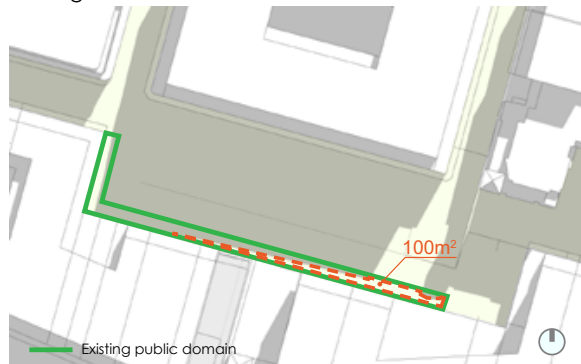
Figure 37 - 100m 2 of sunlight in public domain areas at Grosvenor Lane on 21 June at 10am
