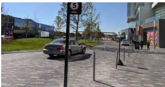
Figure 25 - A shared zone can restrict vehicle access to a space at specific times, allowing the space to be fully pedestrianised periodically.
