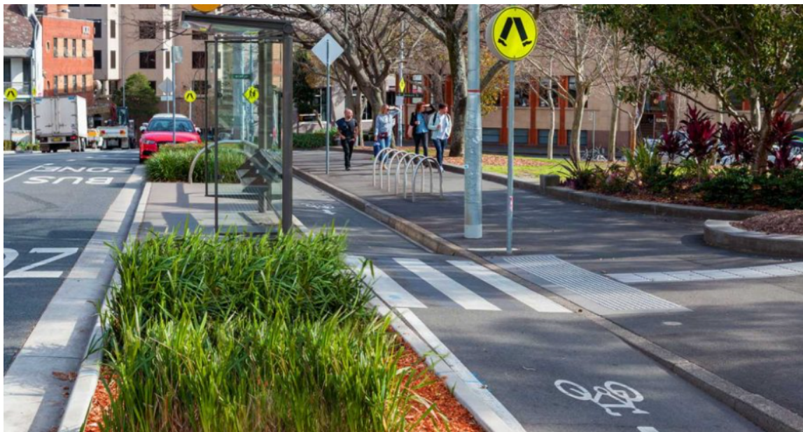
Figure 9. Separated cycle path and bus platform using a similar layout to that initially proposed on Broughton Street.
