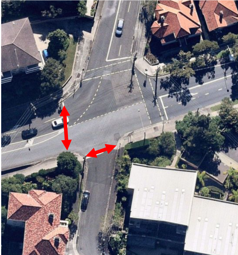
Figure 6. Aerial phot of the intersection between Ben Boyd Road and Kurraba Road showing the location of missing pedestrian crossing legs.
