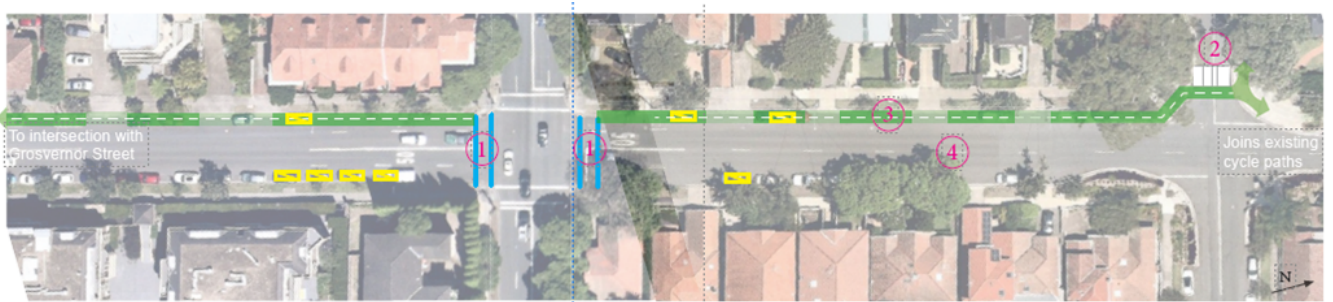
Figure 8 Layout plan showing key project features (yellow boxes indicate loss of parking space locations because of traffic signal upgrade)
