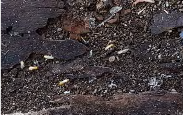
Termites found in timber marine structure
