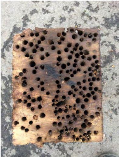
Termites found in timber marine structure
